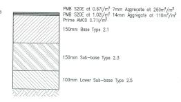
Pavement designs are based on 1000 vehicles per day with 40% heavy vehicles. Geotechnical report prepared by Core Consultants.
